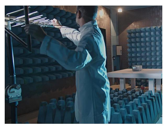
INTEK's advanced instrumentation allows for precise **testing of safety components (SIL)**. The laboratory is equipped with a fully equipped SIDT FAR **anechoic chamber** for 3-meter measurements, ensuring maximum accuracy in evaluations. Additionally, INTEK has a Siemens + Matsushita shielded room to conduct measurements of conducted radiated emissions and disturbance power. The anechoic chamber is designed with a fume and exhaust gas extraction system, ideal for testing small
